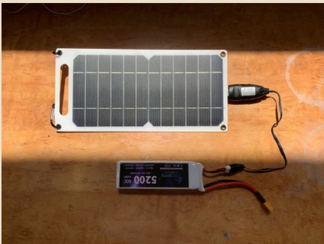
Solar panel for charging the drone's battery
