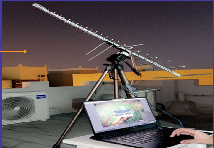
Testing the designed antenna in outdoor environment
