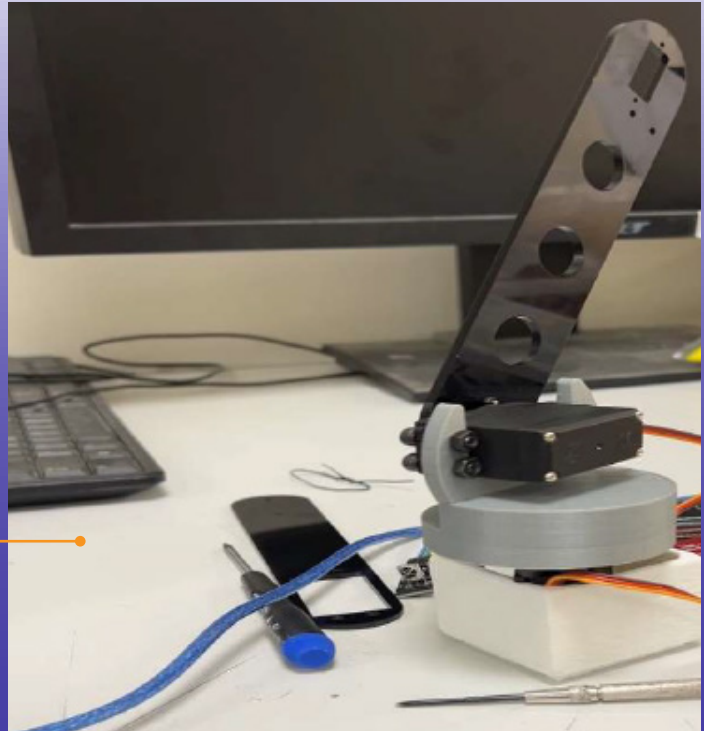
Controlling Device for Antenna Rotation
