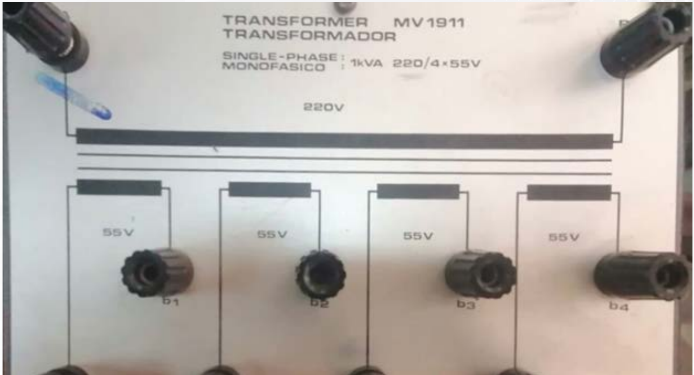
Single phase transformer
