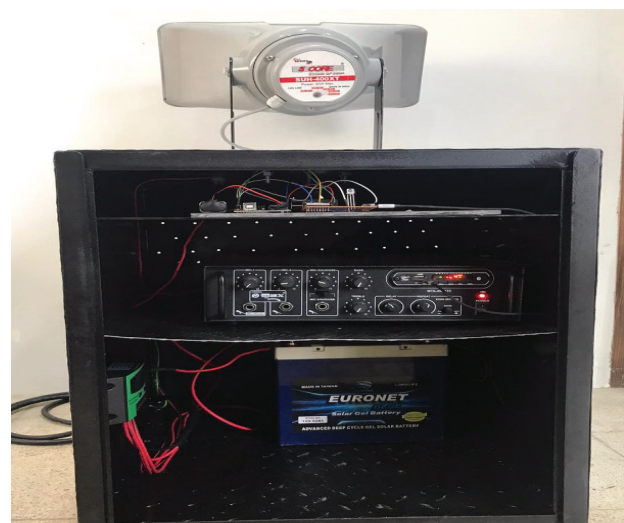
Enclosure of BHMS A box is designed to enclose all electronic components and facilitate the transportation of the prototype.
